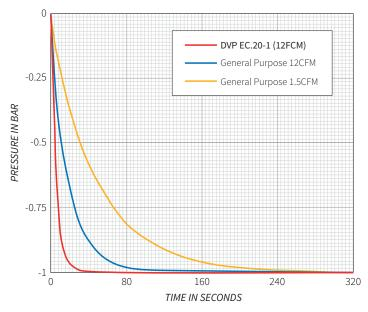
Controlled test conditions. Pressure recorded in empty 26L vacuum chamber.
