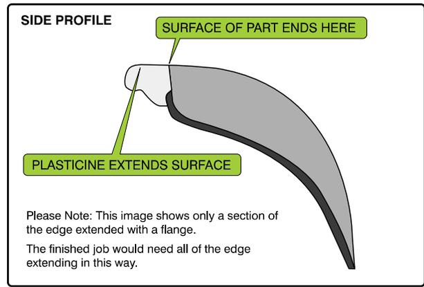
For larger parts it is sometimes easier to use strips of plastic affixed to the edge of the part, secured from the inside, to extend the edges rather than Plasticine.
