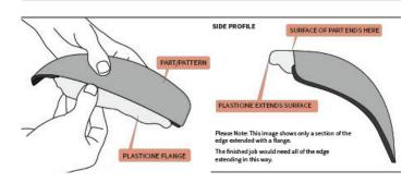
For larger parts it is sometimes easier to use strips of plastic affixed to the edge of the part, secured from the inside, to extend the edges rather than Plasticine.
