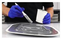
The gelcoat can then be brushed over the surface of the pattern at a thickness of around 0.5mm, try and aim for an even coverage and reduce pooling where possible.
