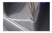
This is easily done by preparing the area with a good key and then adding a small quantity of EG160 tooling gel. Once cure this can be sanded and polished to blend back into the surface of the mould.
