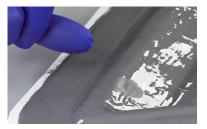
The first gelcoat application should now be left for around 2-3 hours to cure to the 'B' stage, at this point the gel will still be tacky but firm enough that it leaves no residue to a gloved finger when pressed onto the surface.
