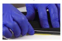
Any gaps between pattern and signboard can be filled with the yellow filleting wax and smoothed out to make a seamless join and prevent any gelcoat from seeping between the two.
