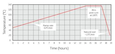
After initial cure, the new mould should be heated - using a very gradual ramp rate to avoid distortion - up to its full service temperature.
