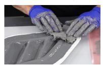
These pieces can then be applied to the mould on top of the wet coupling coat. Care must be taken at this stage to ensure no air pockets are trapped between paste and gel or in the paste itself.
