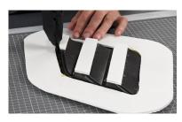
The first step is to add barriers around the perimeter of the shape using a sheet of fluted signboard, when working with prepregs, these flanges can be fairly narrow (around 30mm) but for other laminating methods you may want to increase their size. Once
