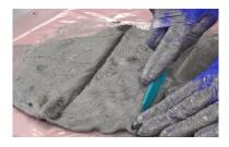
EMP160 & hardener then need to be weighed out and mixed and kneaded for round 2~3 minutes to ensure that the 2 parts are fully combined into a dough like material with consistent texture.
