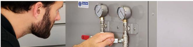
OV301 includes two integral ports which can be supplied complete with optional gauge and valve assemblies for convenient connection of one or two separate vacuum lines into the oven.
