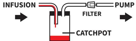
The most common cause of damage to vacuum pumps in composites is ingestion of resin, which can occur in a single major event or can accumulate over time. Always use an inline catchpot and filter when using the pump with liquid resin.
