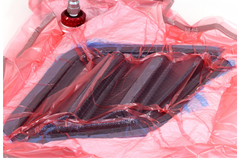
Once laminated, the part is vacuum bagged and cured in an oven at 120°C under vacuum.
