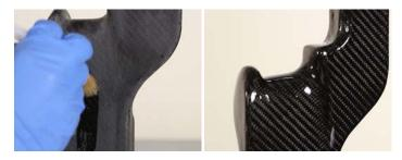
The final layer of resin only needs to be applied very thinly, almost like applying a varnish or lacquer to the part. The smooth surface underneath should make it possible to achieve a smooth, level gloss finish which looks good even before it is flatted and polished.
