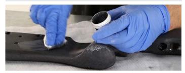
The NW1 Black Super Cutting Compound included with the Skinning Starter Kit and also available separately from Easy Composites should be used to polish the skinned part from a smooth but satin-finish 1200 grit finish up to a full gloss.
