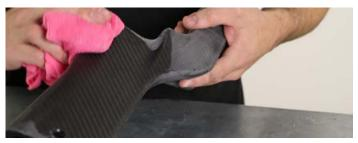
Before applying the final coat of clear resin it is very important to remove all sanding dust from the surface of the part because any dust that remains on the surface when the final coat of resin is added can contaminate the resin and will visible in the final finish. This can be achieved using a tack-rag, microfibre cloth or by washing the part in mildly soapy water.
