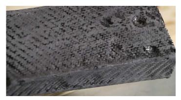
Next you'll need to key the whole surface of the part with more 120 grit paper so that the next layer of resin can bond to it. Whilst you can do some light 'flatting' at this stage (to remove high or low spots in the resin) be careful not to break through to the carbon fibre. If you see the sanding dust turn black then you should stop right away.
