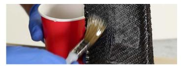
Apply an even coat over the whole surface of the part, making sure you fully wetout the dry carbon fibre. You are never aiming to achieve a thick coat of resin with any single application; instead, thickness is built up using a number of thin layers.
