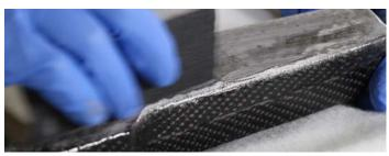
Once the clear layers of resin have cured to a fully hard finish there will now be enough thickness of resin to allow the surface to be properly flatted.
