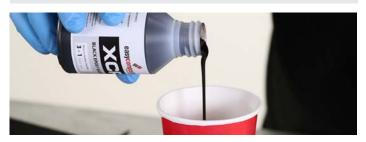
Mix a quantity of basecoat suitable for the size of the part that you are going to skin. To help you to work out the correct amount of basecoat, you'll need about 330g of basecoat (and hardener combined) to cover 1sqm of surface - this means that if you are using the whole of the 0.3sqm of carbon fabric included in the small skinning kit you would want to mix up around 100g of basecoat; if you used half this much fabric then you would only need 50g of mixed basecoat.
