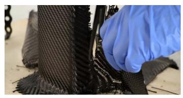
For complex parts you may need to consider completing the surface in multiple sections. With skill, join lines like this can be achieved very discreetly, especially when positioned on corners where they can be almost impossible to see. If you do need to achieve neat join-lines on your part then an epoxy compatible spray adhesive such as Easy Composites' FusionFix<sup>™</sup> is required.
