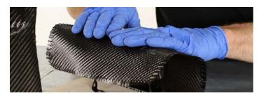
Providing that the basecoat is at the ideal tack level (previous section), it should provide the perfect tackiness for the carbon fibre fabric to stick too.
