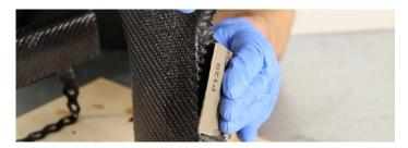
Once the 1st coat of resin has cured to a hard, sand-able finish, use a piece of 120 grit abrasive paper to remove any nibs (often caused by loose fibres at the edge of join-lines standing up), drips or other high spots.
