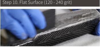
Once the clear layers of resin have cured to a fully hard finish there will now be enough thickness of resin to allow the surface to be properly flatted.
