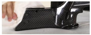
The NW1 compound can be used by hand or with a polishing pad and power polisher. Where available, a power polisher is likely to be much quicker than hand polishing.
