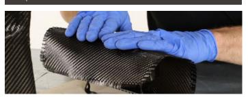
Providing that the basecoat is at the ideal tack level (previous section), it should provide the perfect tackiness for the carbon fibre fabric to stick too.
