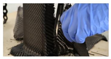
For complex parts you may need to consider completing the surface in multiple sections. With skill, join lines like this can be achieved very discreetly, especially when positioned on corners where they can be almost impossible to see. If you do need to achieve neat join-lines on your part then an epoxy compatible spray adhesive such as Easy Composites' FusionFix™ is required.
