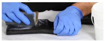
Starting with the 400 grit abrasive paper, wet-sand the surface to a flat smooth finish. Once you are happy there are no high or low-spots, wipe down the surface, change the water and move on to the next grit.
