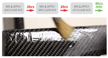
You must NOT allow the previous layer of resin to cure past the 'tack' stage before applying the next layer of resin. If you do, the new layer of resin will not be able to bond properly to the previous layer and could delaminate. You will also find that the new layer of resin will visibly 'fish-eye' away from the previous layer if it is no longer at the tack stage (see recovery method below).
