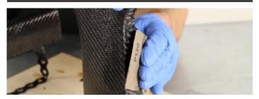
Once the 1st coat of resin has cured to a hard, sand-able finish, use a piece of 120 grit abrasive paper to remove any nibs (often caused by loose fibres at the edge of join-lines standing up), drips or other high spots.
