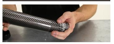
Carbon fibre fabric is very delicate. Even the process of removing the carbon fibre from the tube or roll can be enough to distort the fabric.
