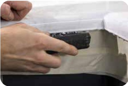
If you find that the front edge has a bit of a 'lip' at the bottom, this can be sanded smooth using increasingly fine abrasive papers, typically 400, 800, 1200, and then finished with a polishing compound such as Pai Cristal NW1.
