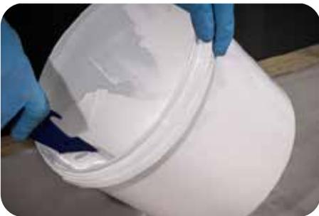
Follow the correct mixing procedure from section 5; it's even more important to make sure you **MIX THOROUGHLY** and **DOUBLE POT** the resin for this main pour following the mixing process on pages 8 & 9.
