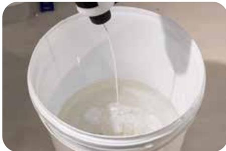
It's fine to add liquid CULR pigments or metallic effect SHIMR powders into the resin before or after you add the hardener. However, because the resin starts curing as soon as you add the hardener, if you want to take your time adding different pigments or effects to the resin, it's better to do this before you add the hardener.
