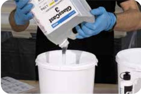
Different resins use different mix ratios, never use the mix ratio for another resin and never attempt to add more or less hardener to speed up or slow down the reaction; that's not how epoxies work. If you are using a GlassCast Countertop Kit then all resin and hardener measurements are done for you; simply weigh out the amounts listed on your kit's 'Colour Card' at each stage of the process.
