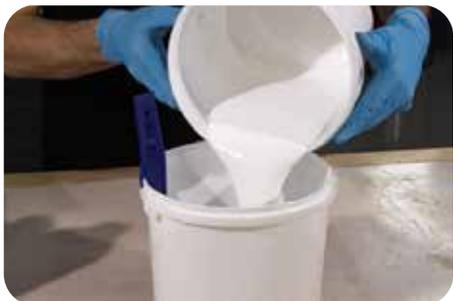
The idea of this process is to ensure that any unmixed resin from the bottom or sides of the pot do not make it out onto your job. This is particularly important when doing the 'main pour' of resin for your countertop as any unmixed resin will not cure and will leave sticky patches or streaks on your otherwise perfect countertop.
