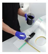
Uni-Mould Tooling Gel Coat should be catalysed at 3% using standard MEKP catalyst. Before application, allow the catalysed gel coat to stand for a few minutes to settle and de-gas.
