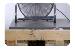
The project is at the upper limit of the 25mm pour, so to air on the side of caution we set up a fan at the end of the workbench to drive excess warm air away from the project and the curing resin and make sure that we keep the temperature of the room around 18-20°C
