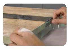
Then apply resin release tape around the entire table top. This will act as a retaining tape around the edge and prevent the GlassCast from flowing off the sides.
