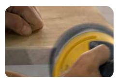
Follow up the trimming by sanding the sides of the table (taking care not to touch the top surface of the slab), work up through the grits from 240 grit all the way up to 1200 grit.
