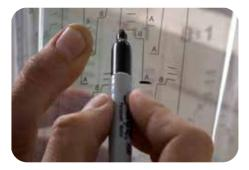
The recommended mix ratio for GlassCast 50 Resin is by volume where the resin to hardener ratio is 2:1, this means 2 parts resin (part A) to 1 part hardener (part B).
