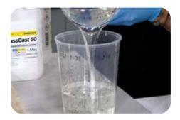
Next pour the mixture into a 2nd clean cup and repeat the mixing process for a further 3 minutes. This process is called double-potting and is to ensure that any unmixed resin from the bottom or sides of the pot do not make it on to the project. If this process is missed it can cause problems to the curing process and the finish.
