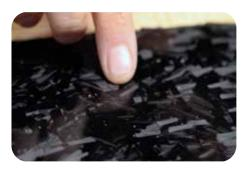
On closer inspection you may be able to see some tiny pinholes, this is difficult to avoid due to the nature of the chopped tow material and can be easily rectified. The next step is optional depending on the type of finish you wish to achieve on your project.
