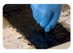
This is because the wood acts as an insulator and if poured too deeply the resin could overheat and lead to problems through overheating. To avoid the possibility of this happening, limit pours to a depth of 25mm and if you require a greater depth of pour you need to allow the first layer to partially cure to the B-stage. The B-stage is where the resin has firmed up but still has a tackiness to the surface - you can test this with a gloved finger - you should be able to make an
