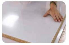
clean surface that the resin won't stick to. Stick the polypropylene sheet down with double sided tape and check that the surface is perfectly level before continuing.
