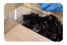
Spread/sprinkle the carbon fibre evenly along the resin river - with the aim of blocking out the surface below with a dense consistent layer.
