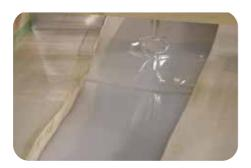
You are now ready to pour the resin into the river! Pour the mixed resin into the river channel, then allow it to stand for a short while to release any bubbles that may be present in the pour from mixing, check the edges to make sure no bubbles are clinging to the sides.
