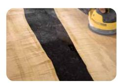
First, flat the surface of the resin to remove any high spots using 120 grit abrasive paper, if you have access to a Dual Action Sander this is the best way to achieve this.
