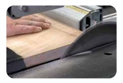
To remove the meniscus left around the edges and neaten the sides of the table, the table top was trimmed on a table saw to take off a few millimetres.
